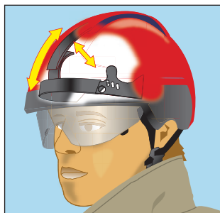
2 The browband position can be easily adjusted up and down, to achieve the best fit between the helmet and the respirator facemask, and any protective hoods
