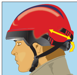
3 The headband size adjustment is easily made by turning a ratchet handwheel which is sized for use by gloved hands and locks in position until released by pressing a central button
