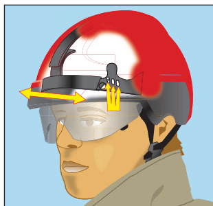
1 The browband position can be easily adjusted between three positions - moving the browband forwards and backwards, to achieve the best fit on the forehead
