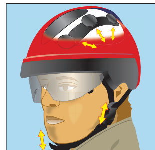
4 The quick release chinstrap can be adjusted for different wearer sizes. Additionally thicker internal crown pads can be fitted if necessary, for small head sizes
