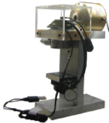
FIGURE 18. Custom ANR Test Fixture with Headset
